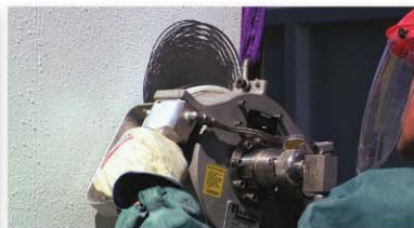
Hand-held VertaJet™ Lightweight, with vacuum recovery
